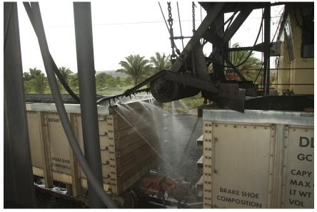
The process of wetting and compacting coal in cars and washing it is also part of the sustainable actions that the company takes to mitigate particle emissions.
