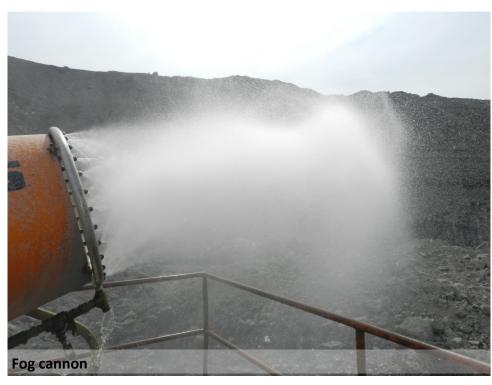
\*To control emissions of particulate matter, Drummond has seven turbine-type fog cannons that operate from the shovel bench to keep dust particles from expanding with the movement of this mining equipment while the trucks are loaded.
