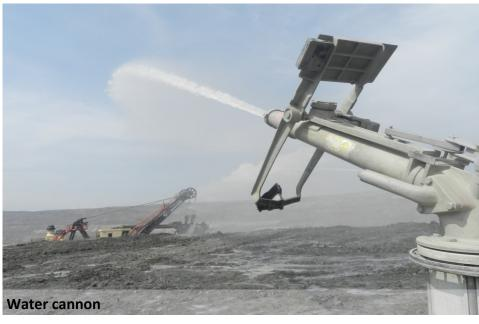
Another one of the sprayers used in the operations is the water cannon. There are 13 of these water cannons that wet the shovel work area with recycled water which minimizes the emissions of particulate matter when the material is loaded.
