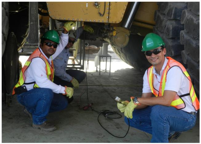
Procedures like measuring the pressure of the trucks' hydraulic lift systems were studied during the course to receive this certification.
